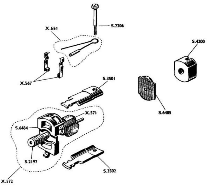
X.500 Complete Motor X.567 Brush Arm and Brush X.571 Armature and Commutator
