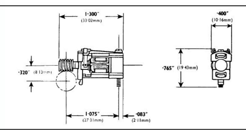
POLES SHAFT DIA. ·0620" (1·575 m.m.) ARMATURE DIA. ... ·375" (9·53 m.m.) ... 0-1 AMP CURRENT ... TWO-START WORM DRIVE REDUCTION RATIO ... 13 to 1 ... ALCOMAX III MAGNET ... ... DELRIN BEARING ... ARMATURE SPEED 20,000 r.p.m.
